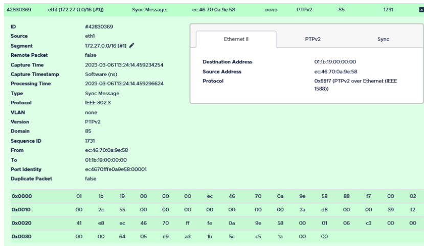
Figure 8.3: PTP Message Breakdown
